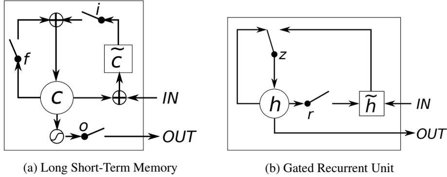
Figure 1: Illustration of (a) LSTM and (b) gated recurrent units. (a)  $i$ ,  $f$  and  $o$  are the input, forget and output gates, respectively.  $c$  and  $\tilde{c}$  denote the memory cell and the new memory cell content. (b)  $r$  and  $z$  are the reset and update gates, and  $h$  and  $\tilde{h}$  are the activation and the candidate activation.
